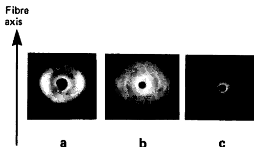
Figure 3 (a) Pinhole pattern of as-spun PET fibre. (b) Pinhole pattern of PET fibre heat treated at T = 140^\circ\text{C} and \sigma = 72 \text{ kg cm}^{-2} . (c) Pinhole pattern of PET fibre heat treated at T = 230^\circ\text{C} and \sigma = 170 \text{ kg cm}^{-2}
